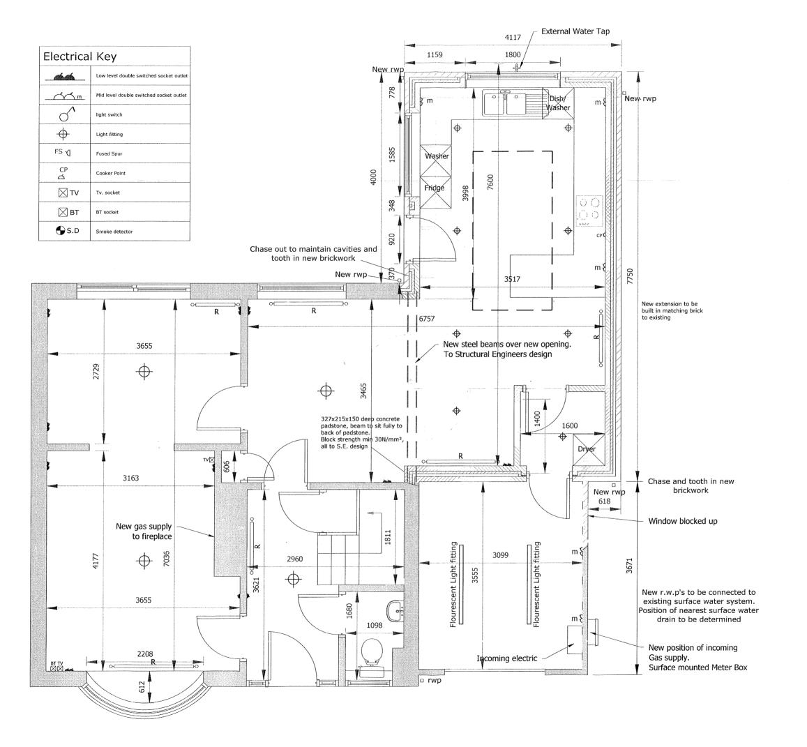
NB | Responsibility is not accepted for errors made by others scaling from this drawing. All construction information should be taken from figured dimensions only
